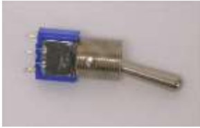
Toggle Switch (Maint/Maint)
