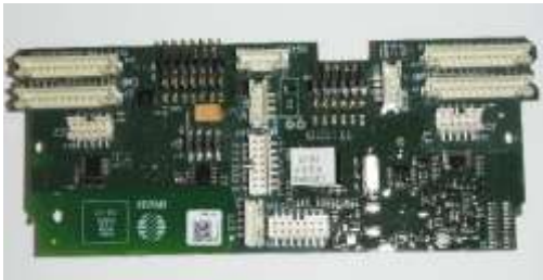
LE72IK EMB Circuit Board (IK2 Console)
